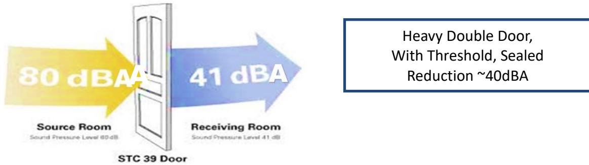
Figure 2.2 : Door usage to reduce noise
